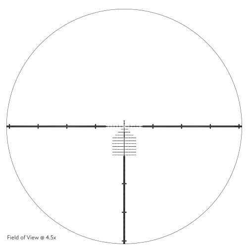
The holdover "Christmas tree" has 0.2 hash marks for distance and windage hold, the numbers for MRAD holdover are placed 1.2mrad on the right from centre to be easily spotted when counting holdover, but still far enough not to cover the target at the most critical parts of the reticle.
